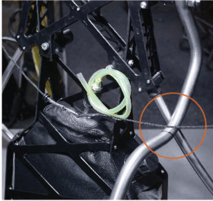
Net-tightening cord carbine position after net is installed to the spars
