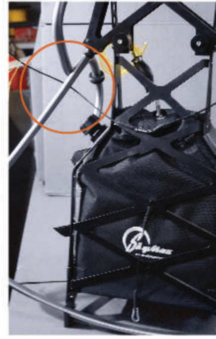
Working position of the net tightening cord and carbine after it is reconnected at the engine side
