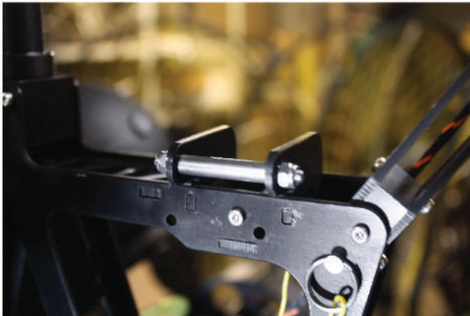
Harness mounting bracket with the stud removed
