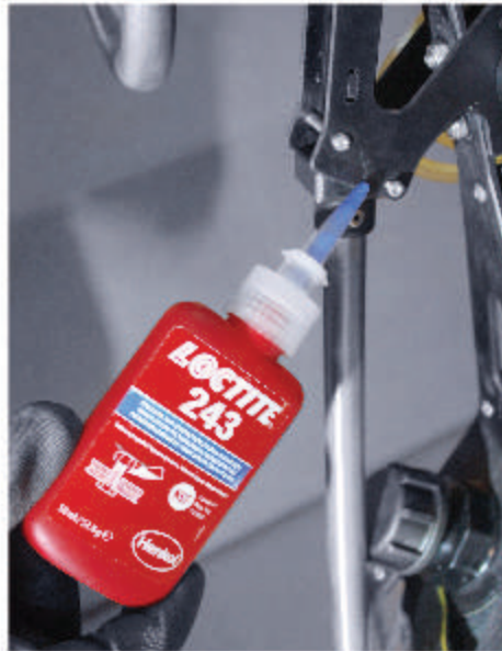
Applying threadlock to the screws
