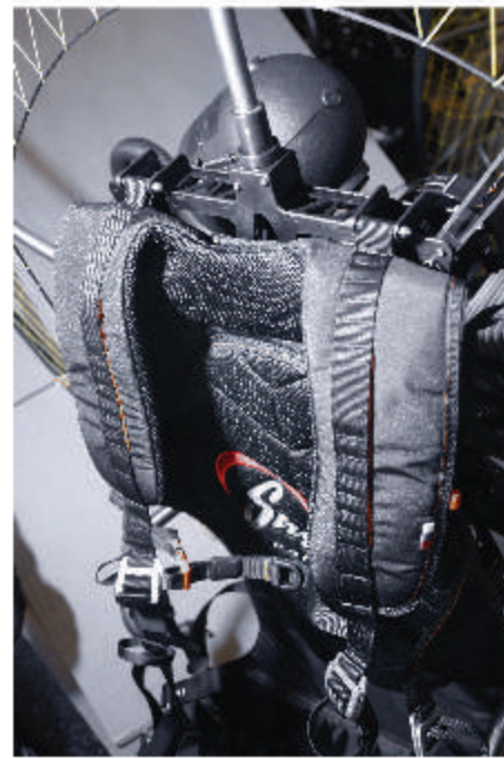
Shoulder straps attached to the frame
