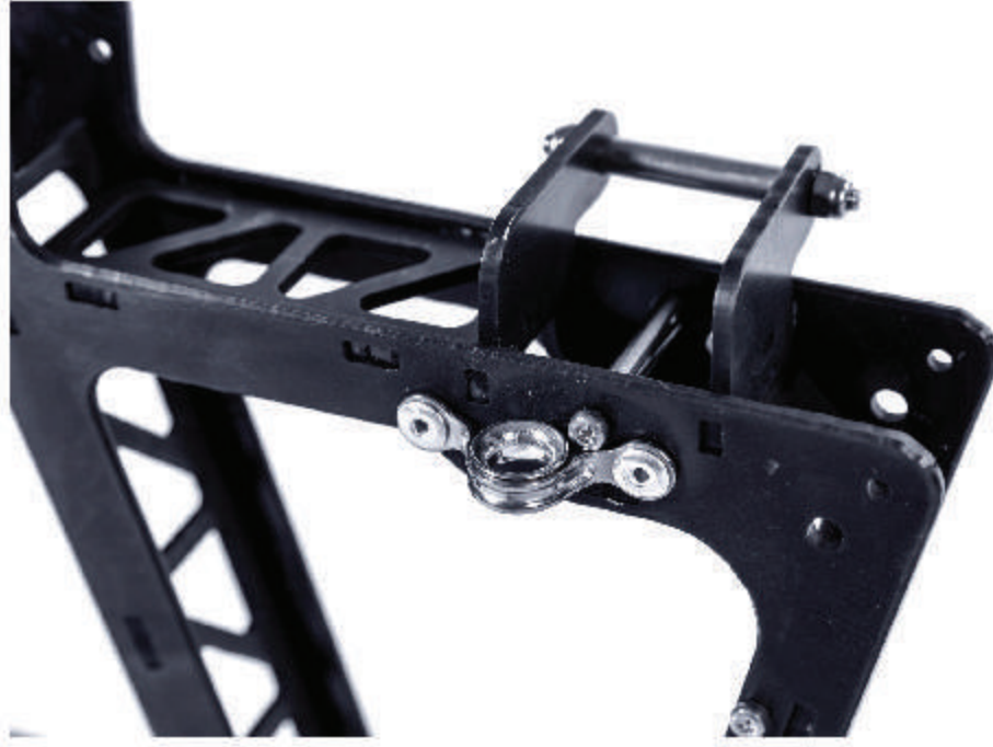
Airbox bracket on the Star frame
