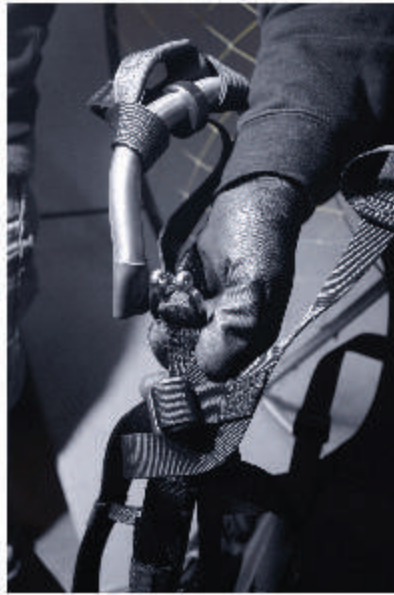
Harness attached to the Ω-shaped shackle
