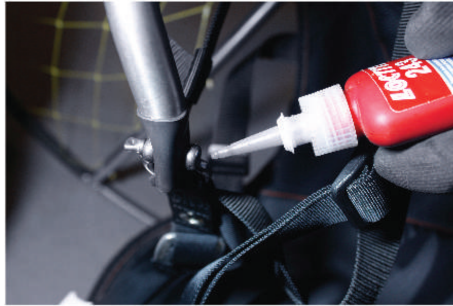
Connecting the harness hang point to S bars
