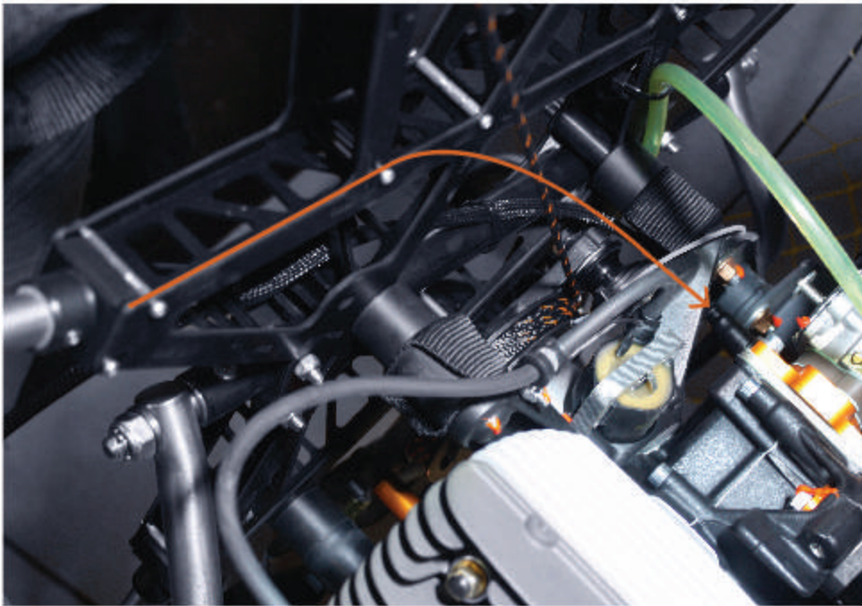
Throttle cable put through SkyMax «Star» frame
