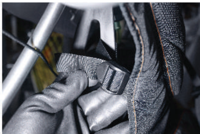
Lower harness strap installation
