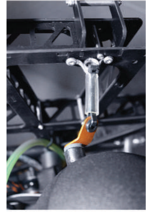
Connecting the airbox to the Star frame
