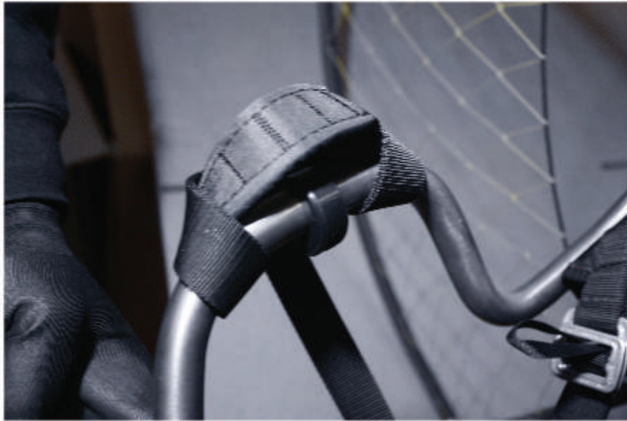
Connecting the harness hang point to S bars
