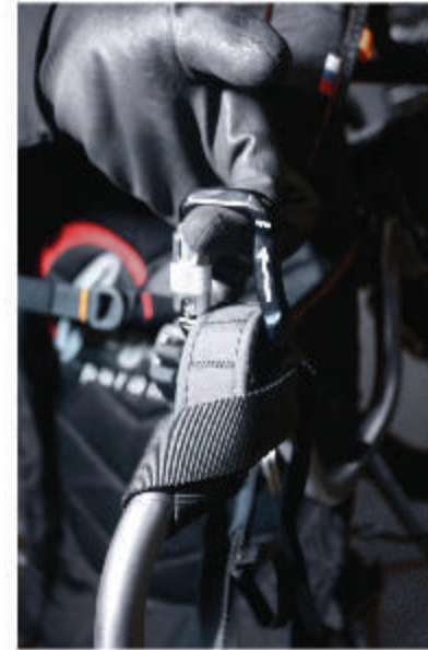
Connecting the harness hang point to S bars
